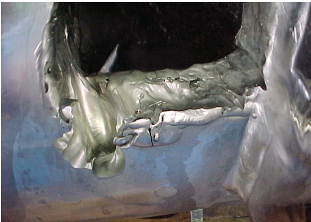
Too high flow created backplash into unprotected drain-zone.
