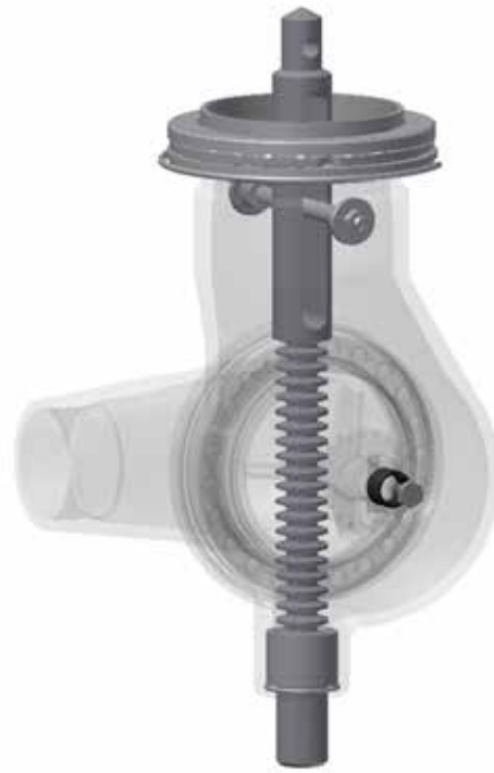
Cleaner head with ball bearings
